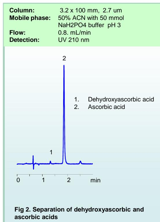
By using mixed-mode columns you can avoid the use ion-pairing reagents for retaining highly hydrophilic acidic compounds. Coresep SB columns have an ion-pairing reagent chemically attached to the surface of the silica gel. There is no need to reserve a column to be used with ion-pairing reagent.
