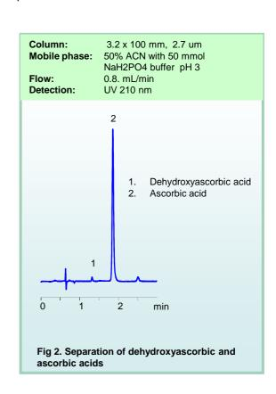
By using mixed-mode columns you can avoid the use ion-pairing reagents for retaining highly hydrophilic acidic compounds. Coresep SB columns have an ion-pairing reagent chemically attached to the surface of the silica gel. There is no need to reserve a column to be used with ion-pairing reagent.
